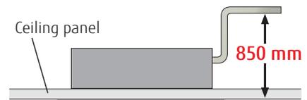
**NEW** Bulkhead Duct Built-in Drain Pump
