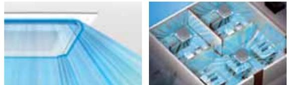
Individual airflow direction control to prevent occupants being exposed to draughts
