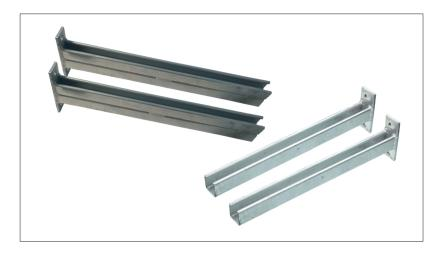
These ready-made, hot-dipped galvanised steel cantilever arms with 14mm diameter holes, offer a quick and easy method of supporting condensing units on external walls. Available in a straight length and webbed version in a variety of lengths. The strut dimensions are 41mm x 41mm x 2.5mm.
