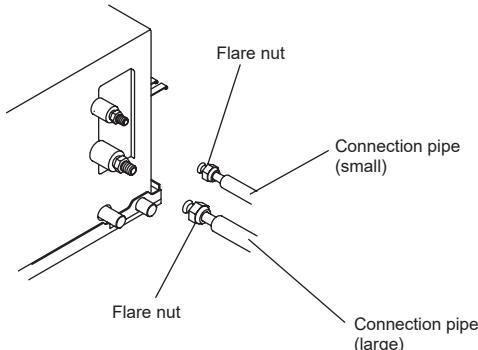
(3) When the flare nut is tightened properly by your hand, hold the body side coupling with a separate spanner, then tighten with a torque wrench. (See the table below for the flare nut tightening torques.)
