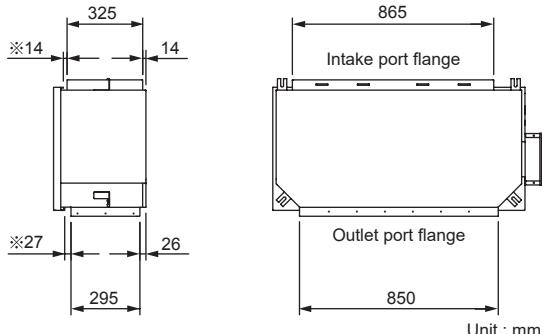
※ Spacing between flange and drain pan.
