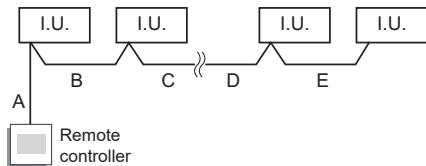
A, B, C, D, E : Remote controller cable. (Refer to "2.4. Electrical requirement")
