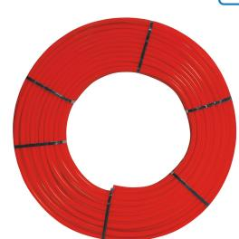
Multilayer EVOH pipe is constructed from flexible, durable raised-temperature polyethylene (PERT). It is further protected by an EVOH oxygen-barrier layer, which prevents oxygen from entering the system and safeguards components such as radiators and valves from corrosion.
