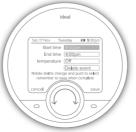
Alter the start and end times of the heating period and the temperature by scrolling and then pushing the dial to edit. Then use the dial to alter the time or temperature and push to confirm. Push the dial or the right hand button to save your changes.
