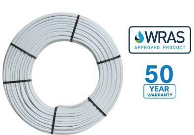
Pert-Al-Pert pipes feature a multi-layer construction with an ultrasonically welded aluminium core. Additional inner and outer layers of PERT II plastic are bonded to the aluminium, resulting in a durable composite pipe capable of operating reliably under combined conditions of 10 bar pressure and temperatures up to 95°C.
