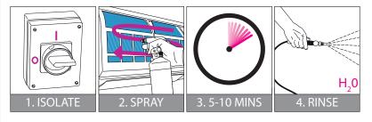
Isolate electrics. Spray into coil, starting at top corner and working methodically across and down. Rinse thoroughly with clean water after use.
