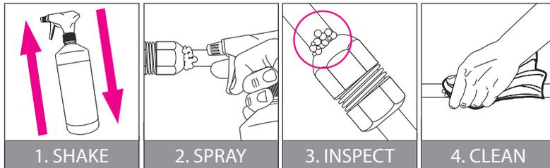
Spray onto suspect joints to achieve an even coating. Large leaks bubble up immediately; slow, small leaks bubble up within a few seconds or minutes. When leak detection has been completed, wipe inspected areas with a damp cloth.
