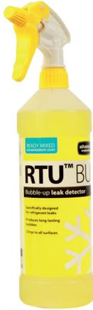
RTU™ BU is a bubble up leak detector which is specifically designed to locate refrigerant leaks. Standard bubble-up leak detectors, designed for use with natural gas, are unsuitable: their lower viscosity means they will not cling to surfaces as effectively and can easily be blown off the pipework before the refrigerant leak is identified.
