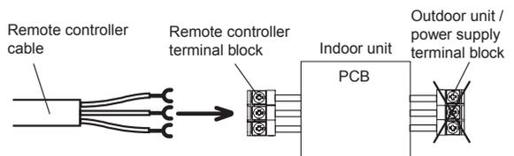
It may be failed if it is connected to the outdoor unit or the terminal block for power supply.
