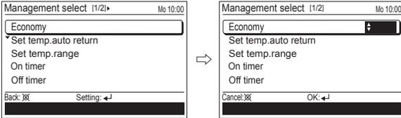
Select the setting with the [Cursor button (Up/Down)], and press the [Enter button].
