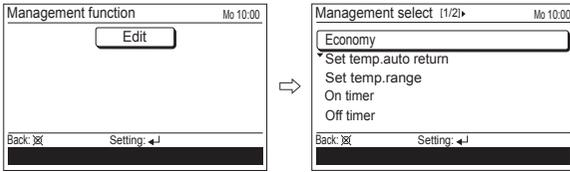
**4** Select the target function with the [Cursor button (Up/Down)] and press the [Enter button]. Then the setting field for the restriction setting is displayed.
