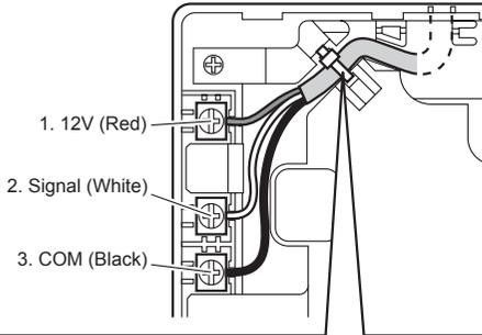
To avoid an excessive tension or pressure to the terminal block, fix the remote controller cable with the cable tie properly.
