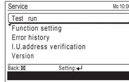
When you select [Test run] with the [Cursor button (Up/Down)] and press the [Enter button], following confirmation screen is displayed.
