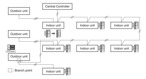
3) Only one refrigerant system is 3-line connection and other refrigerant systems are 2-line connection:
