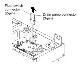
Insert the supplied short-circuit connection to the place where the connectors were removed.
