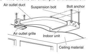
Check to make sure the unit is installed in a horizontal position by using a level.
