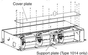
2. Attach the cover plate and the support plate removed in Step 1 and filters (accessories) in the direction shown in the figure below.
