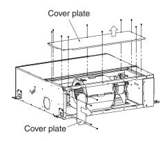
2. Attach the cover plates removed in Step 1 and filter (accessory) in the direction shown in the figure below.
