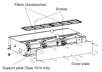
3. Attach the filters (accessories) in the manner shown in the figure. Securely fix the filters with the screws.
