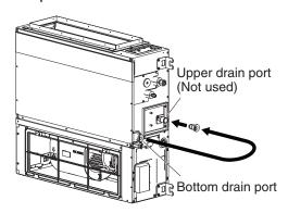
The drain cap can be inserted easily by using a screwdriver or similar tool to push the drain cap into the drain port on the main unit. Push the drain cap into the main unit's drain port until it reaches the end-stop.
