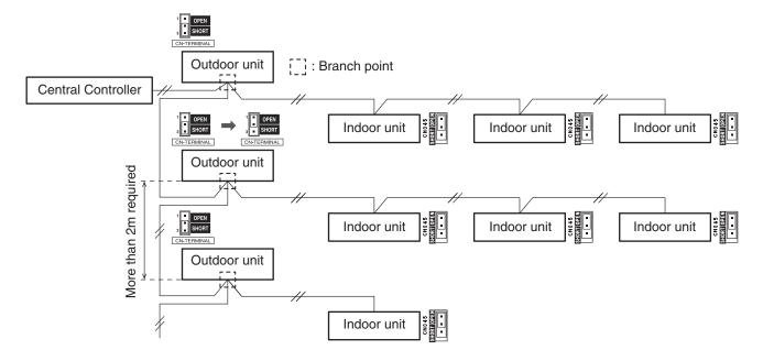
2) Only one refrigerant system is 2-line connection and other refrigerant systems are 3-line connection:
