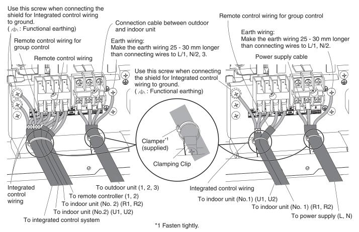
After all of the wires are connected, close the lid of the electrical component box. Make the distance between two cables (1) and (2)) as shown in the figure to the right.
