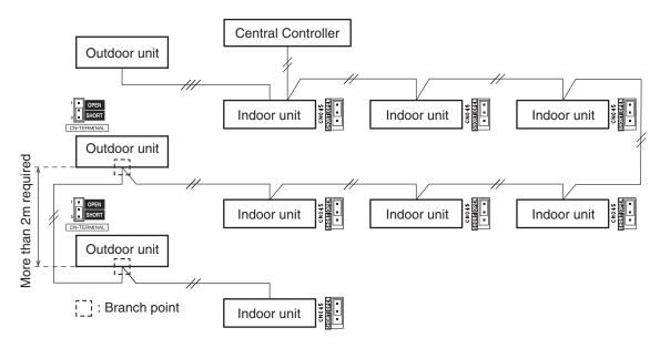
(5) Use shielded wires for inter-unit control wiring (C) and ground the shield on both sides, otherwise misoperation from noise may occur. Connect wiring as shown in Section 4-3.
