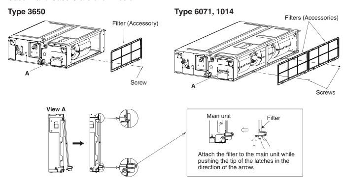
Attach the filters (accessories) in the manner shown in the figure. Securely fix the filters with the screws.
