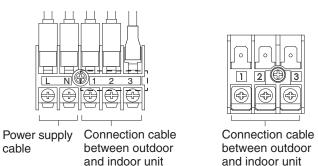
The examples above show the outdoor unit terminal boards. Carefully refer to the outdoor unit installation instructions.
