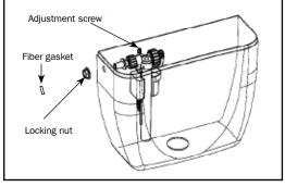
3 - Do not use connector handling the internal part of the inlet valve.
