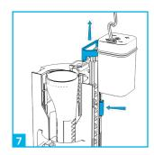
Clip battery compartment into the adjustable holder. Adjust it's height to ensure clearance from the water by pressing button and lifting the rod.
