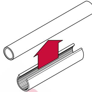
Push the open side of the cover onto the pipe. Snappit Cover will flex and snap into position to grip the pipe.
