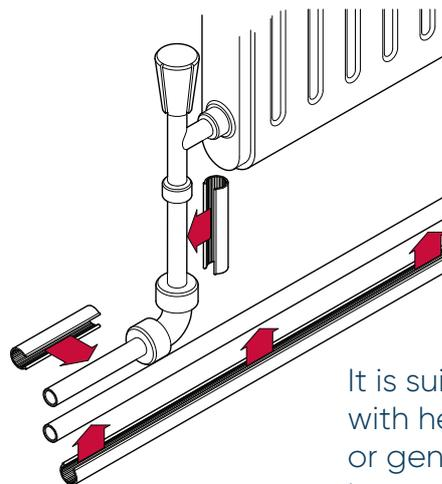
Snappit Cover is compatible with plastic or copper pipe.
